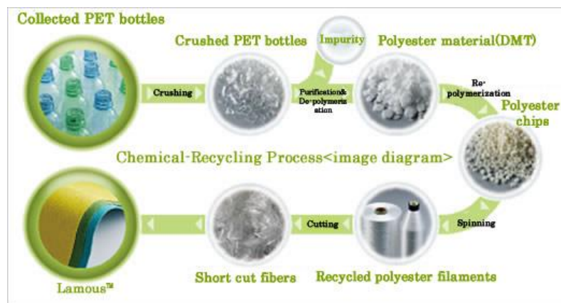
Figure 48: The process for recycling the polyesters [24]
